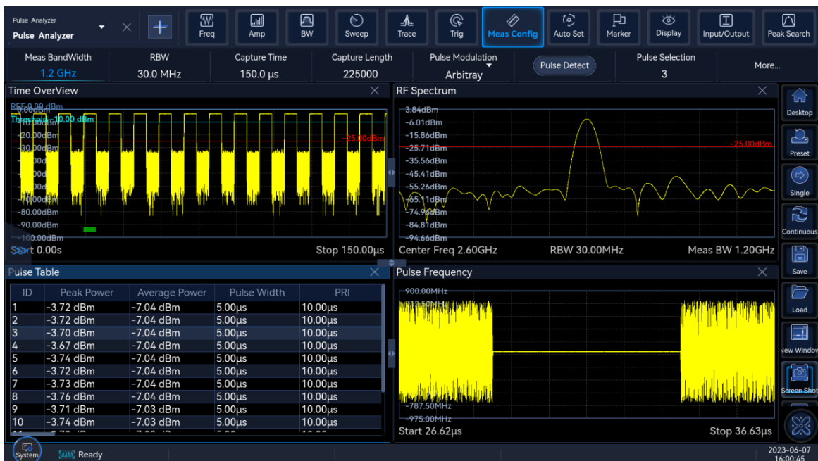
1.2GHz Analysis Bandwidth Measurement
