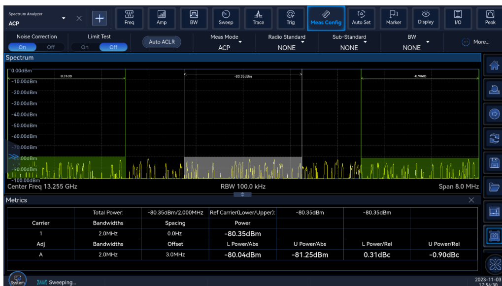
Adjacent Channel Power Measurement Screen
