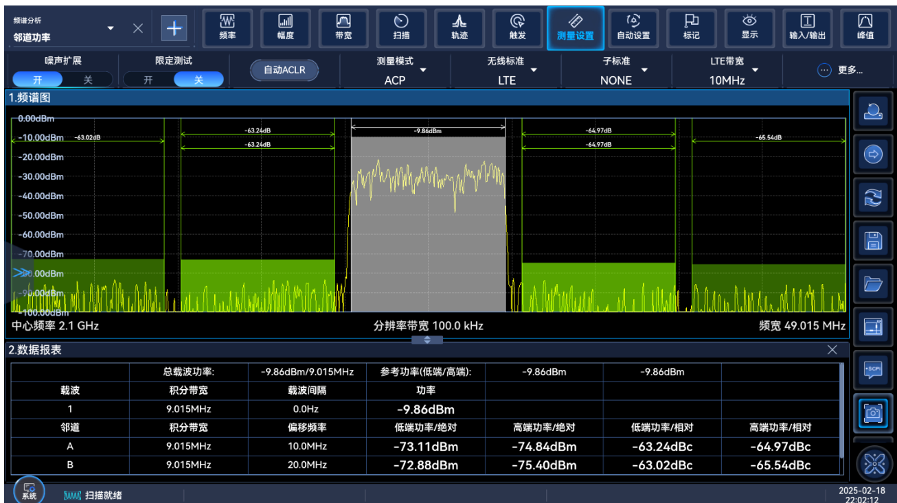
ACLR Measurement Results (LTE, 10MHz LTE E-TM3.1,2.1GHz)
