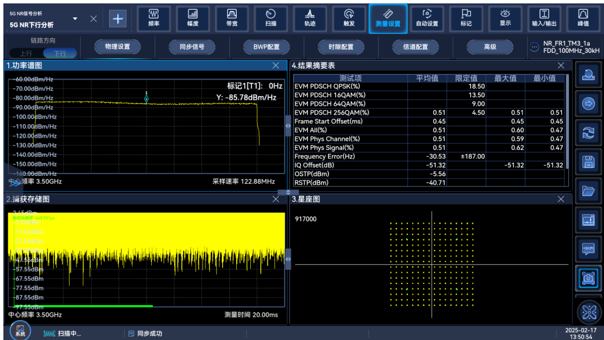
EVM Measurement Results (5G NR FR1, 100MHz, 256QAM, 30kHz SCS, 3.5GHz)
