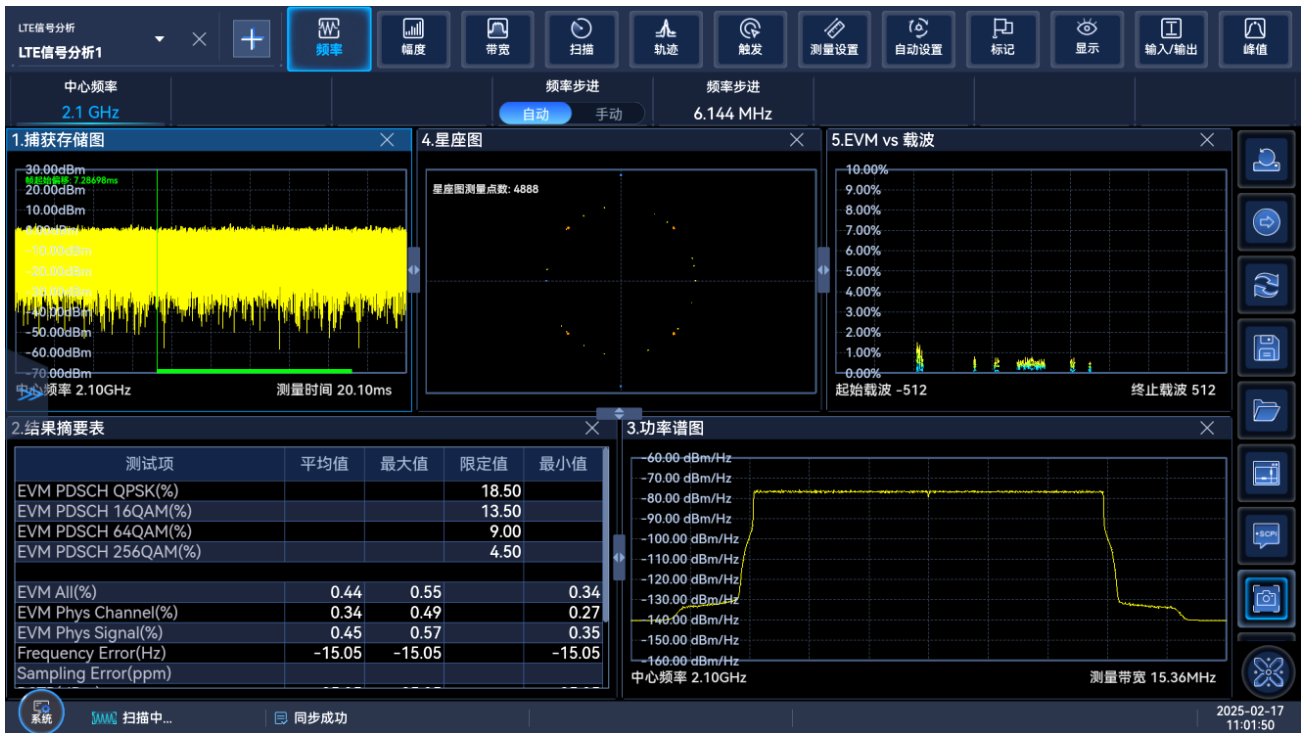
EVM Measurement Results (LTE, 10MHz LTE E-TM3.1,2.1GHz)
