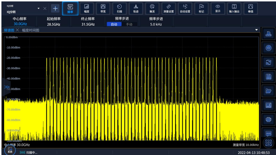
30GHz carrier 2GHz modulation bandwidth multi-tone signal spectrum
