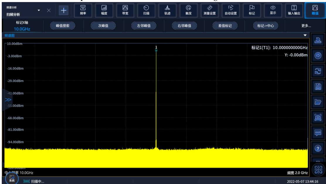
10 GHz carrier spurious test results
